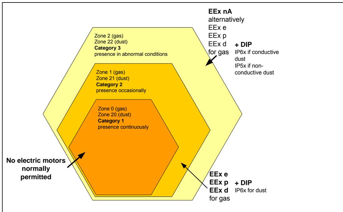
**Figure 7-1 Permitted Equipment Categories for different hazard levels**
